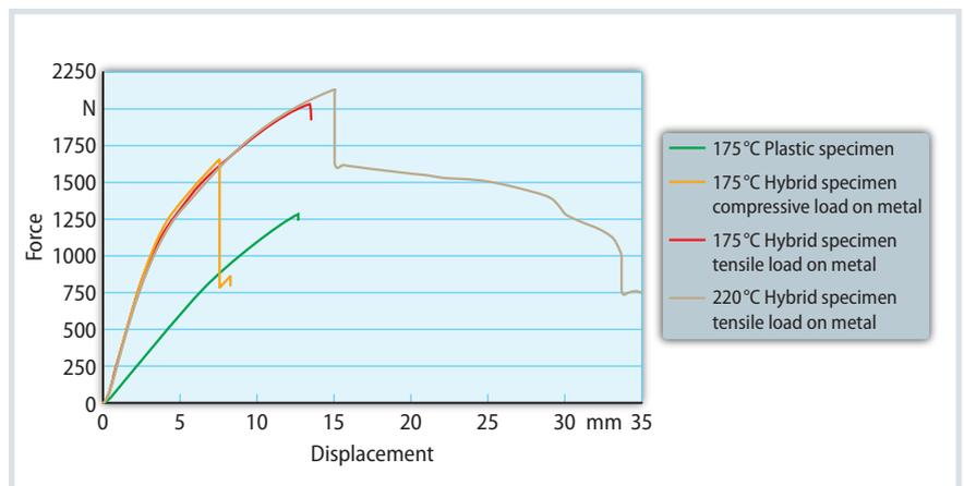
**Fig. 4.** Force-deformation chart of the tested specimens. The hybrid structure increases the stiffness and strength compared to plastic-only test specimens Source: Akro-Plastic/Yizumi; graphic: © Hanser
