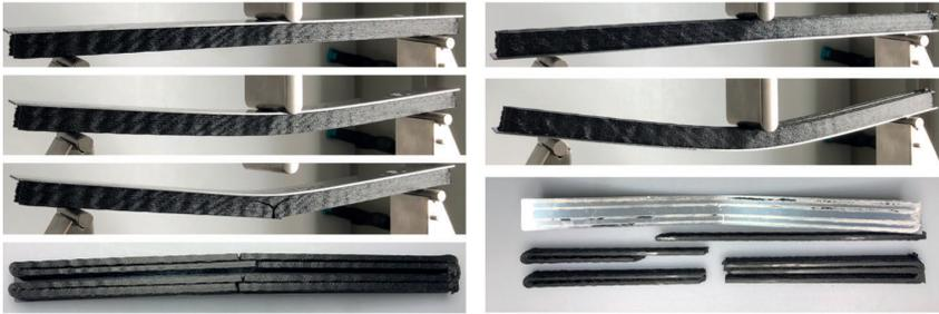
**Fig. 5.** Testing of the hybrid part: initial position (force applied to the metal component on the left, force applied to the plastic component on the right), maximum deflection of the test specimen and failure with fracture mode (insert temperature 175 °C) © Akro-Plastic/Yizumi
