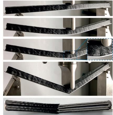
**Fig. 6.** Test in starting position (force application to the plastic component), maximum deflection of the test specimen and failure with fracture mode (insert temperature 220 °C)
