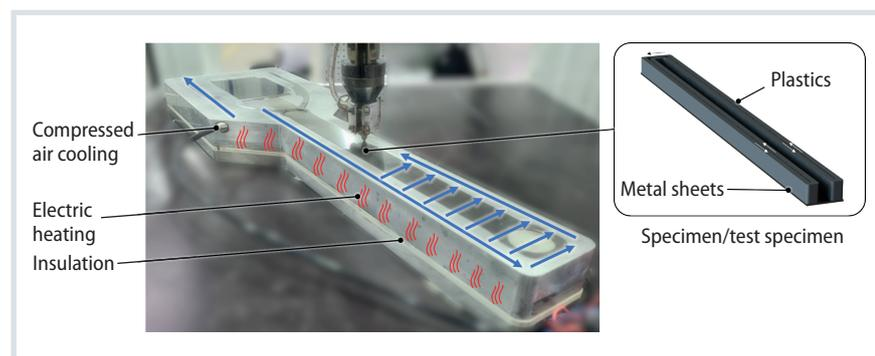
**Fig. 2.** Test set-up: variothermal fixture in production area of a SpaceA manufacturing unit, temperature load cycle and test specimen geometry © Yizumi
