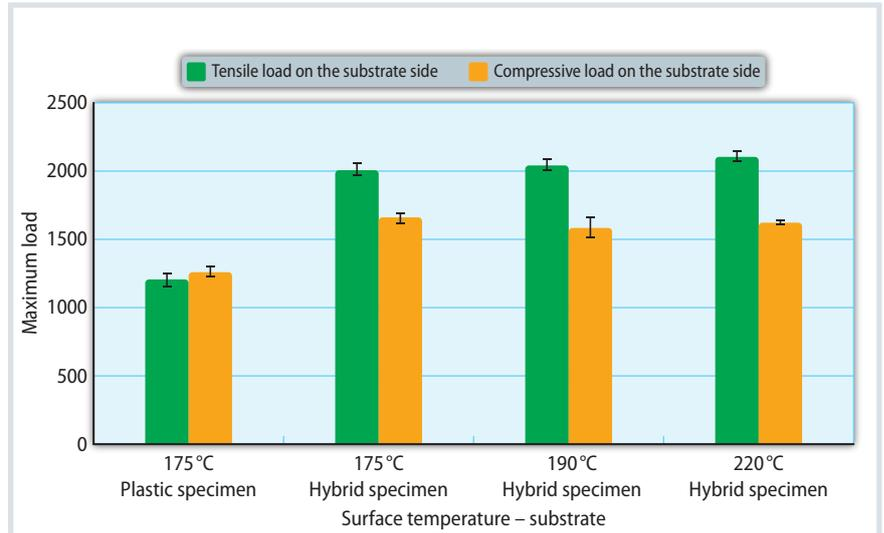
**Fig. 3.** Maximum load at different insert temperatures. This demonstrates the strong bond between plastic and metal over a wide temperature range Source: Akro-Plastic/Yizumi; graphic: © Hanser
