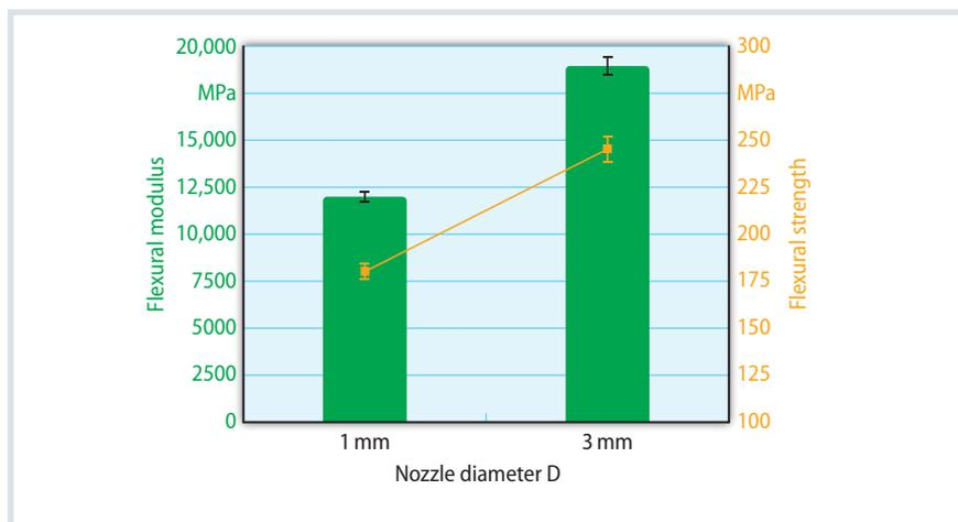
**Fig. 1.** Increasing nozzle diameters have a positive effect on the anisotropy of mechanical properties in the part Source: Akro-Plastic/Yizumi; graphic: © Hanser
